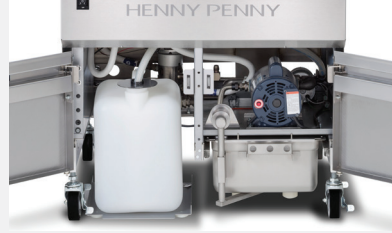
Flex lines throughout with easy access to selector valve and filter pump
