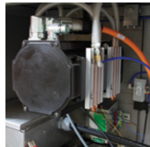
No maintenance direct drive train, zero backlash.
