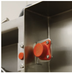
Coded safety interlocking sensors.
