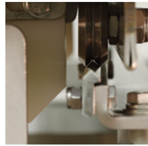
V-groove roller bearing, moveable table.
