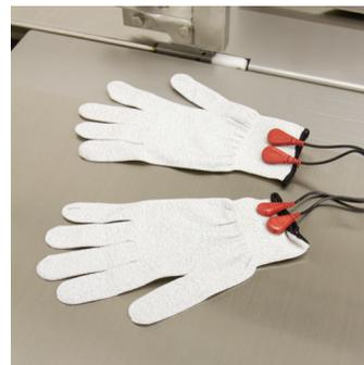
**Color detection Gloves.** Special cotton or rubber gloves worn by the operator are verified before every start up to ensure proper P.P.E. is being worn.
