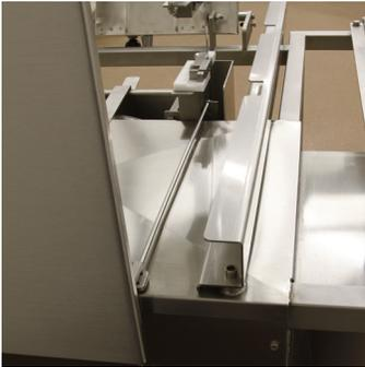
**Water Spray pre-attached blade cleaning system.** Provides continuous and efficient blade cleaning.
