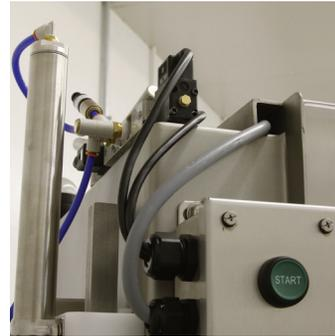
**Pneumatic Auto Blade Guard.** When the saw is stopped the blade guard automatically lowers reducing the risk of inadvertent contact with a stationary blade.
