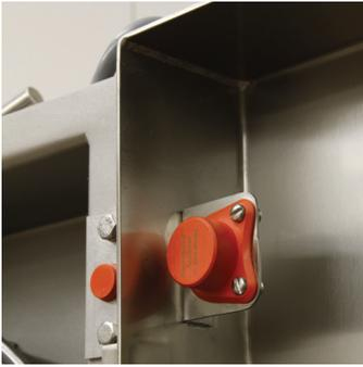
**Coded safety interlocking sensors.** Braking system immediately engages when either the upper wheel door or lower wheel door are opened.
