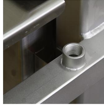
**Frame clean-out flushing port.** Stainless steel construction, with built in flushing ports, for ease of cleaning.
