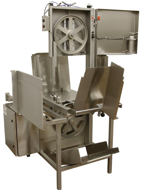
**Swing open hinged table and door design** provides superior cleanability. All components stay attached to the saw which minimize the loss and damage of parts.
