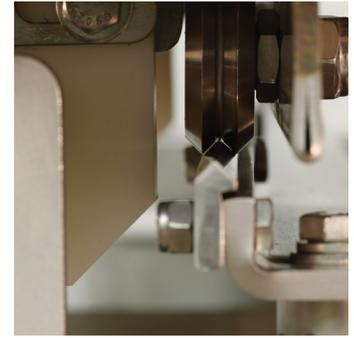
**V-groove roller bearing, moveable table.** Smooth and solid table roller design maintains positive product tracking with stainless steel roller bearings.
